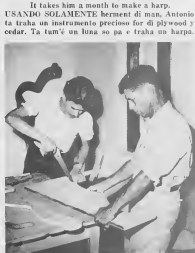
USING ONLY hand tools, Antonio constructs an instrument of beauty from plywood and cedar.
